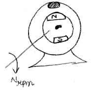
Pate of change of flux linkage occurs in conductor which produces dynamically inducted emf.
